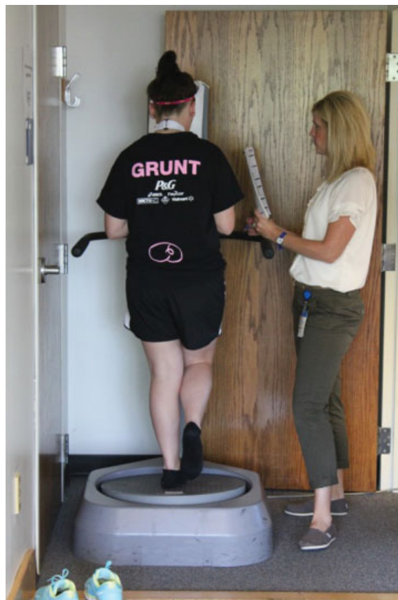
Fig. 3 Assessment of dynamic unilateral postural stability task using a stabilometer from which proprioception and coordination measures were calculated.
